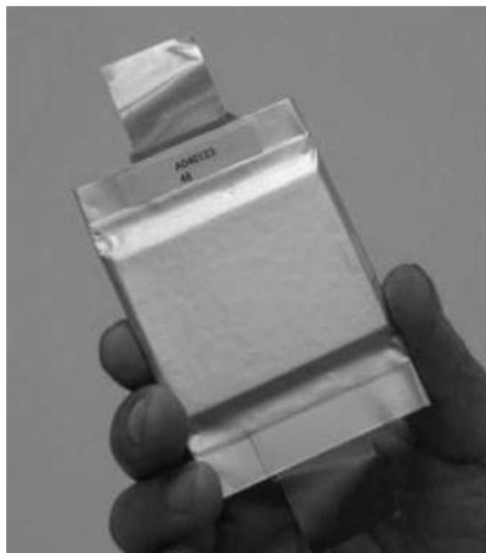
Fig. 1. An appearance of an Al-laminated film packaged organic radical battery.
